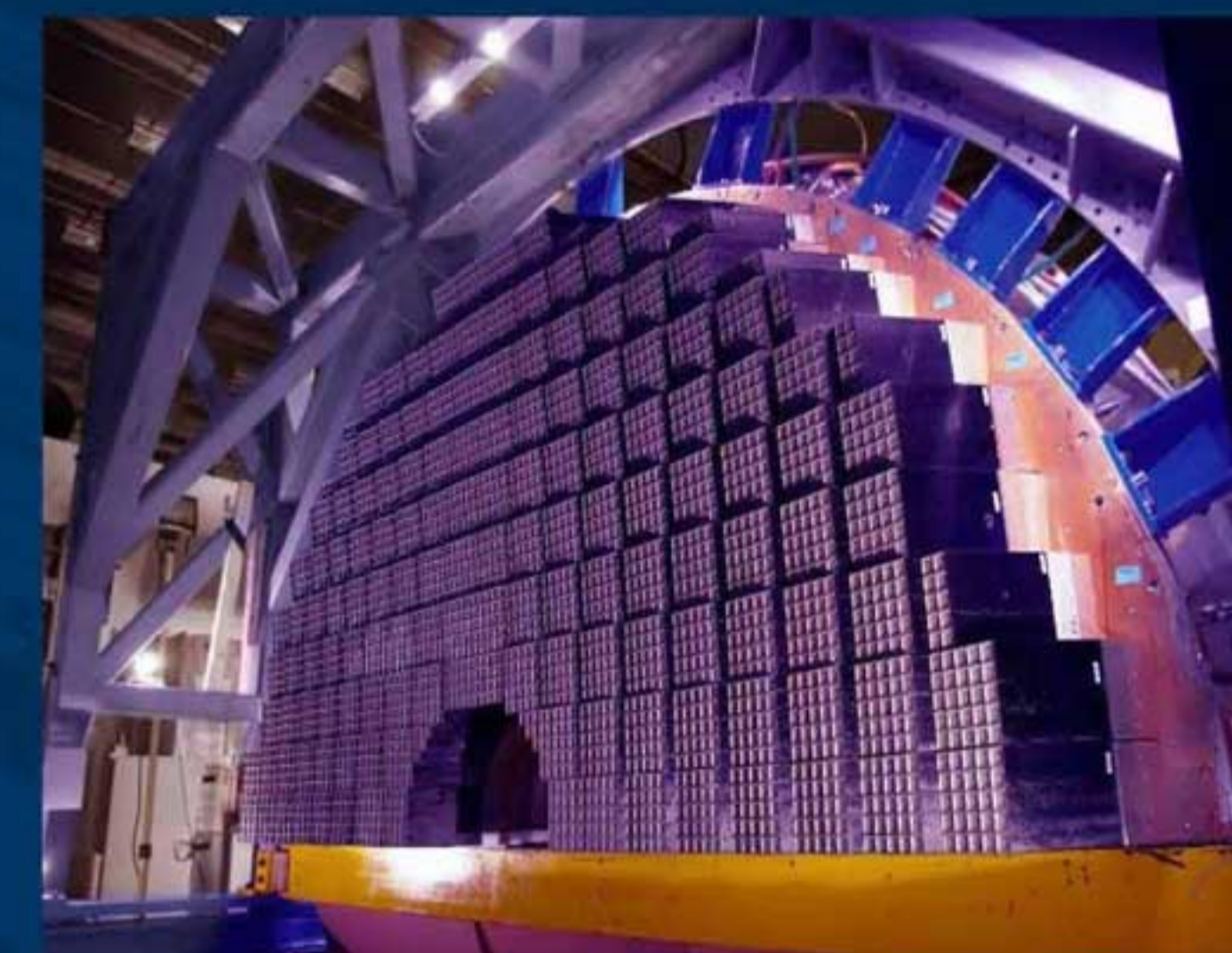
The CMS electromagnetic calorimeter detects high energy photons and electrons. RAL led the design and construction of its "endcap", shown here.
