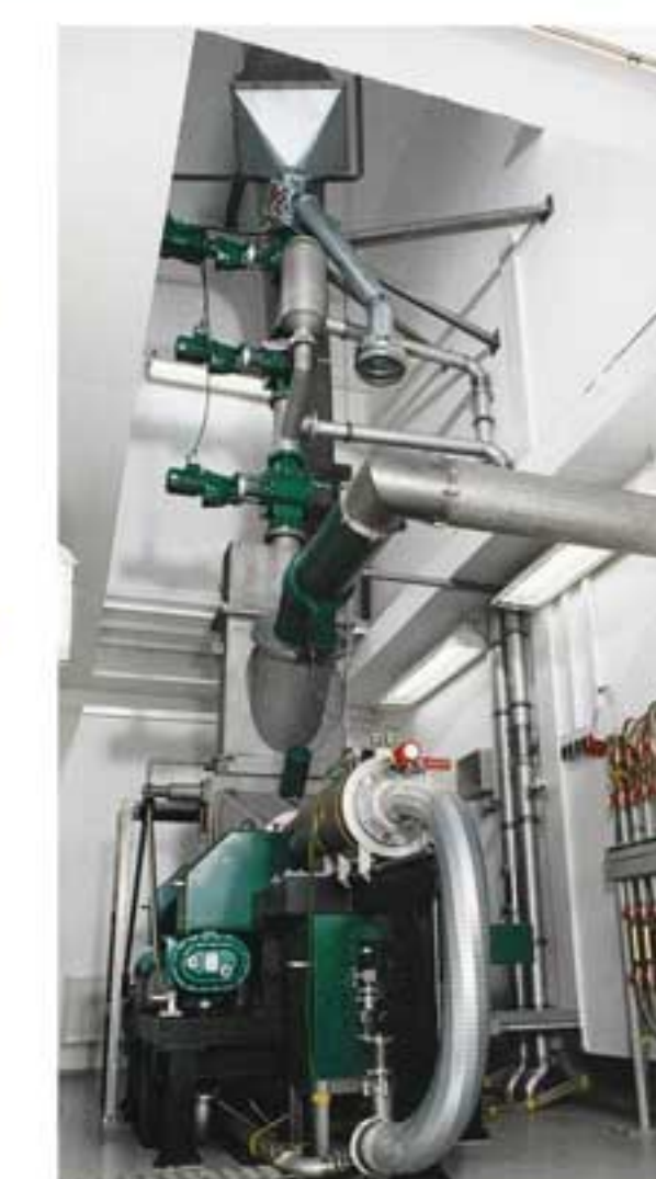
Electron beam facility in Germany for treating seeds
