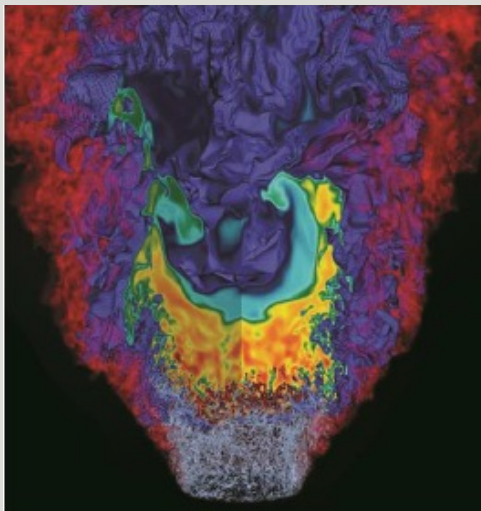
Figure 6 - A computer simulation of the spatial distribution of N 2 O, NO and OH species in a hydrogen flame.
