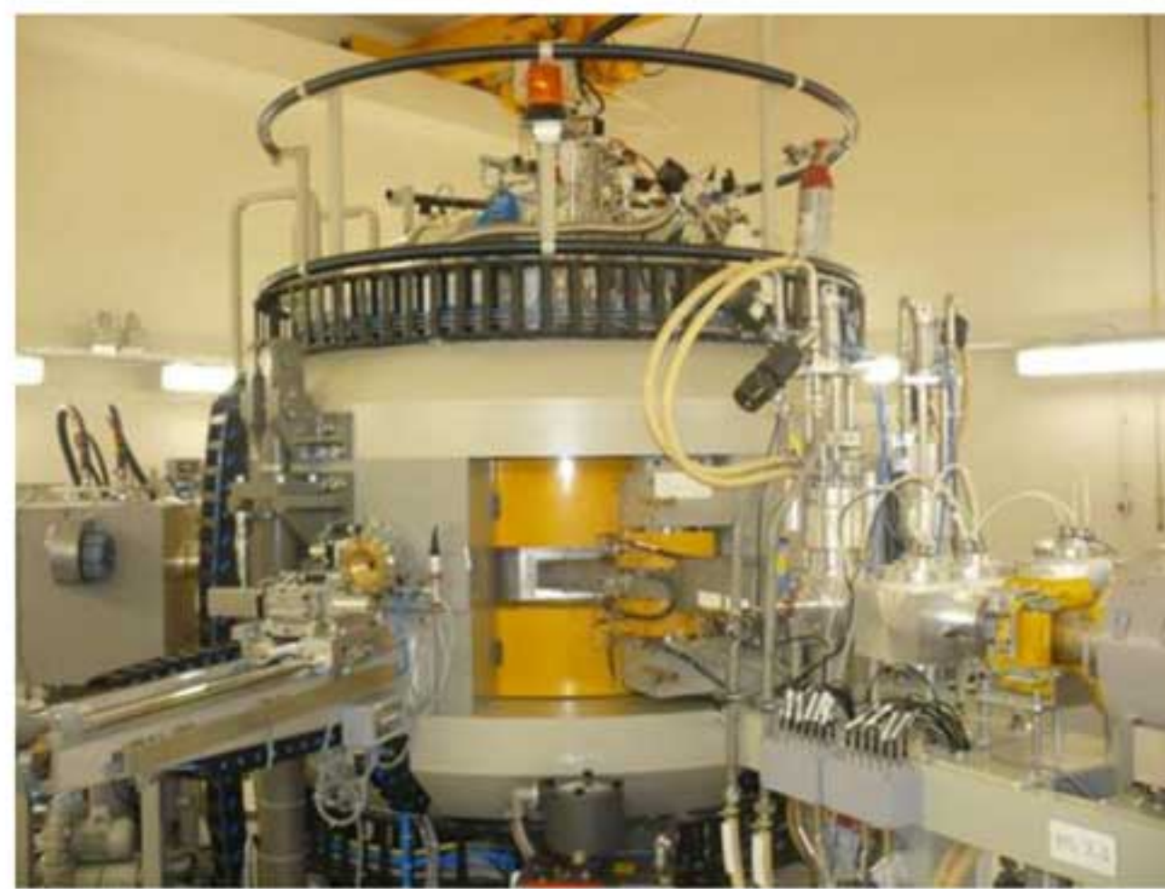
A 30 MeV radioisotope production cyclotron manufactured by IBA of Belgium
