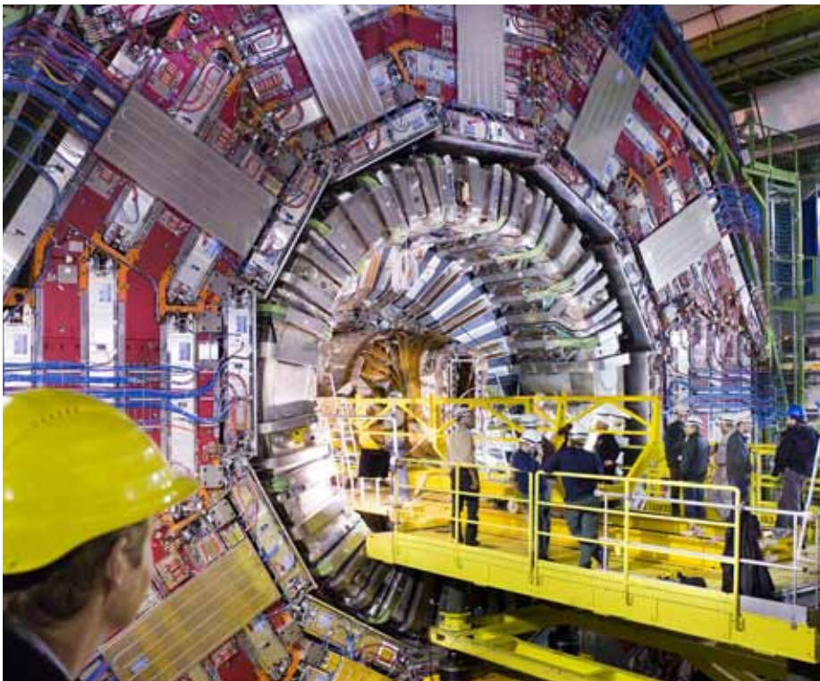
The tracker is inserted into the centre of the CMS detector. (Credit: CERN)
