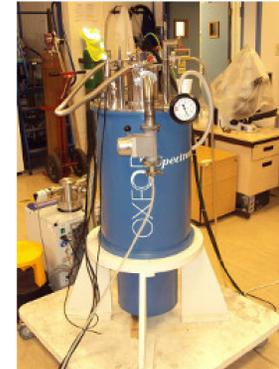
7 T large bore cryomagnet (Cambridge)
