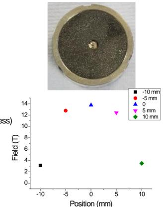
In Cambridge we can apply fields up to 7T. However the sample's peak trapped field remains at 7T until it warms up to above 50K. This implies that single stage portable cryocoolers which can reliably reach that temperature would be suitable for creating portable 7T permanent magnet devices at our facility.
