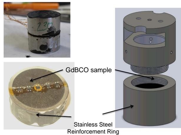
Two bulk samples mounted in stainless steel rings with thermally conductive epoxy resin sandwich hall probes between the two top surfaces. The gap between the top surfaces is <1mm. In addition to 10 or 15% Ag in the bulk we add a silver heat sink core through the centre of the sample axially to allow for maximum heat removal.
