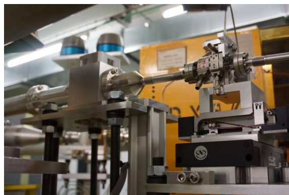
Jack's BPM (top right) being put through its paces in the CLIC Test Facility © J Towler
